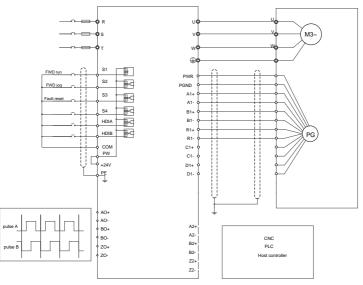
**Note:** If the connected encoder does not have CD signals, you do not need to connect the C1+, C1-, D1+, and D1- terminals of the PG card.
