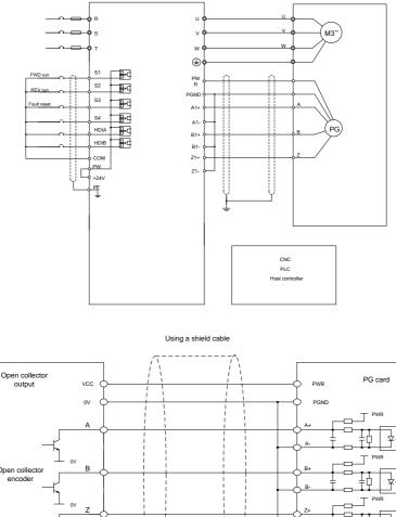
Figure E-31 External wiring when used with an open collector encoder
