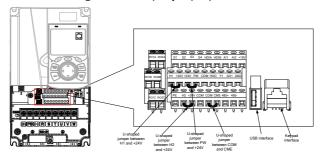
Figure 4-9 U-shaped jumper position
