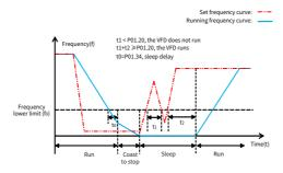
When the set frequency is lower than the frequency lower limit, and the ones place of P01.19 is set to sleep, the VFD stops according to the tens place of P01.19 and sleeps once running at the lower limit for the time specified by P01.34. If the set frequency is higher than the lower limit once again and it lasts for the time specified by P01.20, the VFD restores to the running state automatically and increases to the set frequency.
