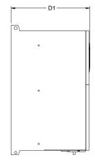
Figure C-5 Outline and mounting dimensions of 380V 132–200kW VFD models
