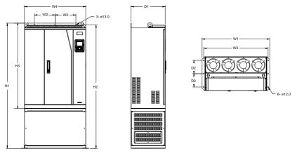
Figure C-12 Outline and mounting dimensions of 660V 400–630kW VFD models
