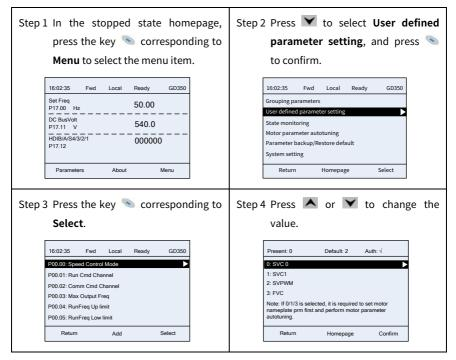
Step 5 Press the key 🛸 corresponding to **Confirm**. The page returns to the user defined parameter list, and you can continue to modify parameters or return to the previous menu. 16:02:35 Fwd Local Ready GD350 P00.00: Speed Control Mode P00.01: Run Cmd Channe P00.02<sup>,</sup> Comm Cmd Channel P00.03: Max Output Freq P00.04: RunFreq Up limit P00.05: RunFreq Low limit Return Add Select
