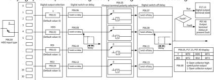
The following table lists the options of function parameters P06.01–P06.04. A same output terminal function can be repeatedly selected.
