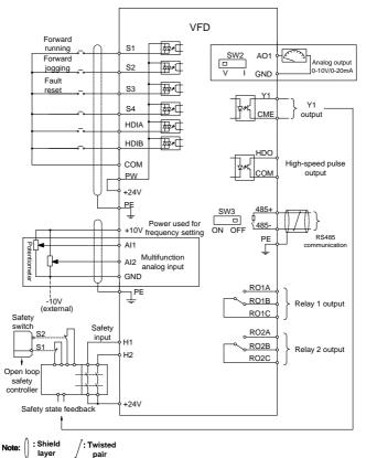
Figure 4-6 Control circuit wiring
