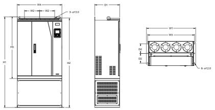
Figure C-7 Outline and mounting dimensions of 380V 355–500kW VFDs
