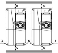
Figure 3-3 Installation space of multiple VFDs
