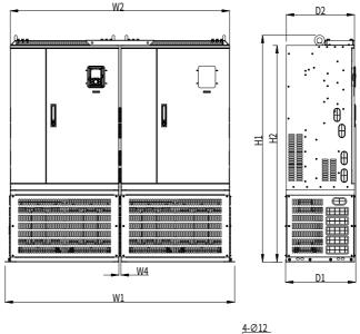
Figure C-15 Parallel outline and mounting dimensions of 660V 710kW VFD models
