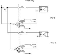
Method 2: If the input signal comes from the PNP transistor, set the U-shaped jumper between COM and PW based on the power used according to the following figure.
