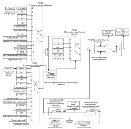
When setting the auxiliary frequency inside the VFD by selecting function 10 or 11 for one function codes from P05.01–P05.06, you can increase or decrease the frequency quickly by setting P08.45 (Up terminal frequency incremental change rate) or P08.46 (Down terminal frequency decremental change rate), as shown in the following figure.
