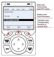
Example of parameters displayed in fault state
