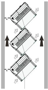
Figure 3-5 Tilted installation space
