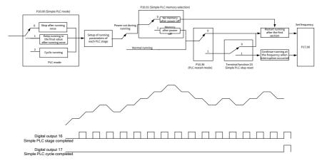
When simple PLC is selected for frequency giving, you need to set P10.02–P10.33 to determine the running frequency and running time of each step. The schematic diagram is as follows.
