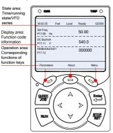
Example of parameters displayed in stopped state
