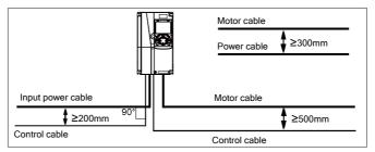
Figure 4-1 Cable routing distance
