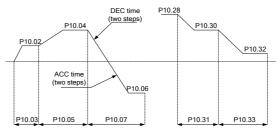
✓Note: The symbol of multi-step speed determines the running direction of simple PLC, and the negative value means reverse running. ACC time indicates the time needed for the VFD to accelerate from 0Hz to the max. output frequency (P00.03). DEC time means the time needed for the VFD to decelerate from the max. output frequency (P00.03) to 0Hz. Select corresponding ACC/DEC time, and then convert 16-bit binary number into hexadecimal number, finally, and then set corresponding function codes.
