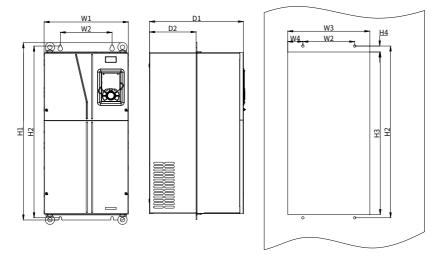
Figure D-7 Flange mounting dimensions and hole spacings for VFDs of 660V 55–132kW
