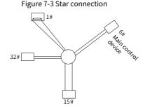
Use shielded cables, if possible, in multi-device connection. The baud rates, data bit check settings, and other basic parameters of all the devices on the RS485 line must be set consistently, and addresses cannot be duplicated.
