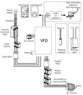
Figure 2-2 System configuration
