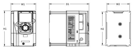
Figure C-3 Outline and mounting dimensions of 380V 45–75kW VFD models
