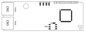
**Note:** For this card, before power-on, set the SW1 switch according to the mapping between protocols and positions.
