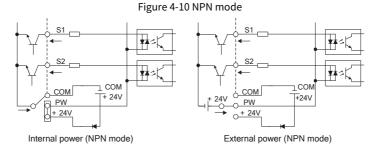
✓ Note: When the internal power is used in wiring mode 1, the S terminals of different VFDs cannot be connected in parallel, as this may cause malfunction of the S terminals. If the S terminals need to be connected in parallel (between different VFDs), a diode must be connected in series between 24V and PW (with the anode connected to 24V). The diode must meet the requirements: IF > 40mA, VR > 40V, as shown in Figure 4-11.
